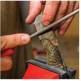
**PRO-TIP:** Use the files to remove any deep scratches you made with the rasp before moving on to sanding.
