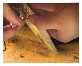
When mounting the handle scales, make sure the holes line up perfectly and the screws enter easily. If the fit seems off, don't force it. Brute force never truly solves anything. Simply remove the scales and sand the edge of the scale that contacts the bolster until you've reached perfect alignment.
