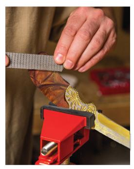
**PRO-TIP:** You'll be shaping the handle with the blade open. 10 out of 10 doctors and mothers advise you mummify the blade in many layers of masking tape to protect yourself while you work.
