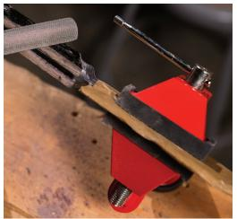
Next, get to work removing the parts of the handle scale not in contact with the knife tang. Use the rasp for all the heavy lifting. Remember when we mentioned your work station would get messy? This is the time and place to make that mess.
