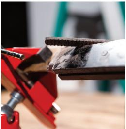
Once you've achieved your desired handle shape, switch over to the mill file, and remove all deep gouges and scratches. The file can also be used to shape the bolster, but be prepared, the hardened steel will require more effort and patience.
