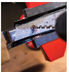
Time to put the "fun" in "functional kitchenware ornamentation" by inserting the mosaic pins. Coat both the pins and pin holes with epoxy, then insert the mosaic pins into the finished assembly. It's okay if the pins protrude from the handle surface. They can be shaped later with the handle.
