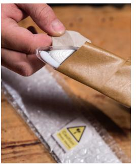
Leave the plastic sleeve on, and use masking tape or some other heavy tape to secure the plastic sleeve onto the blade. This will protect both your fingers from the knife, and the knife from the tools that you'll be using to make the handle.
