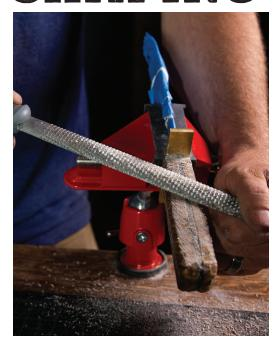
**PRO-TIP:** The brass guard can also be shaped with the same hand tools. Rounding the corners and tapering the handle along the length can make it more comfortable and more functional.
