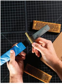
Let's take a dry run and assemble the handle of the knife. We'll start with the guard. Slide the brass guard onto the handle until it's flush with the guard stop. If the fit is tight, you may need a hammer or mallet to tap the guard into place.
