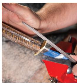
Remove any excess material that hangs over the tangs until the knife profile is flush with the steel tang. Now, it's time to maximize comfort and character. Keep removing material until it feels comfortable in your capable, knifemaking hands.
