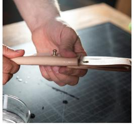
Take care to line up the sheath's outer edges as flush as possible. The glue doesn't require clamping, but you should use your hands to press the two pieces together for about a minute to allow the glue to set.
