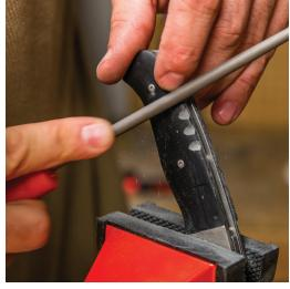
The Micarta is made of layers of linen encased in a hard plastic. As you work through layers, it will reveal a wood grain pattern. You can use the fine files to create unique patterns and grips for you handle.
