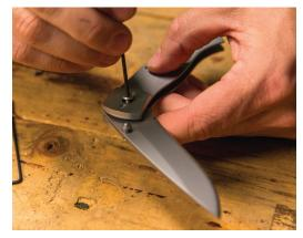
When mounting the handle scales, make sure the holes line up perfectly and the screws enter easily. If the fit seems off, don't force it. Brute force never truly solves anything. Simply remove the scales and sand the edge of the scale that contacts the bolster until you've reached perfect alignment.
