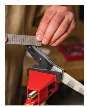
**PRO-TIP:** You'll be shaping the handle with the blade open. 10 out of 10 doctors and mothers advise you mummify the blade in many layers of masking tape to protect yourself while you work.
