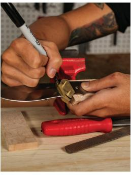
Sand the ends of the pins to remove any burrs, and assemble the bolster. Mark the shape and design onto the bolster, then remove and re-assemble without the blade. Using the vise and files, roughly shape the bolster to your design.
